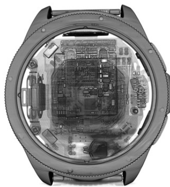
3D microCT scan of intact smartwatch. 1x1 image for web.
