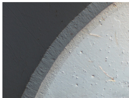
This image shows a thermal spray coating, imaged with C-DIC contrast. (Coating cross-sections)
