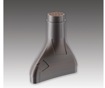
Figure 1: FDM sacrificial tooling begins with a 3D printed tool, which features a standard fill pattern designed to promote fluid flow during the tool removal process and provide adequate strength during elevated temperature, high pressure cure cycles.
