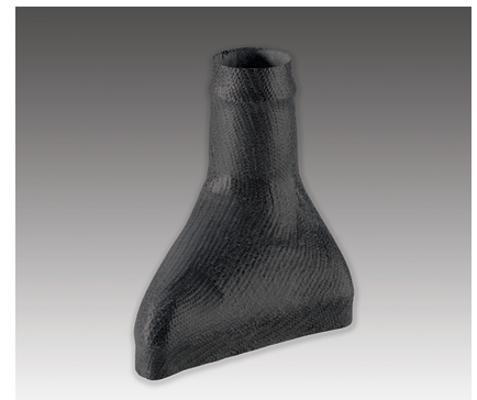
Figure 3: The FDM tool is easily removed, hands free, leaving the final composite part.
