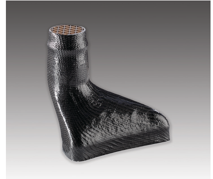
Figure 2: The composite material is then wrapped around the sacrificial tool as shown. Once the part is fully formed and cured, the tool is ready for wash-out.
